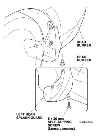
14. While holding the left rear splash guard against the rear bumper, tighten the four self-tapping screws in the order shown.
