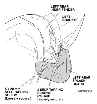
13. Loosely secure the left rear splash guard to the rear bumper with one additional 5 x 20 mm self-tapping screw provided.
