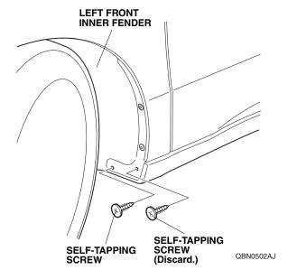
4. Loosely secure the left front splash guard on the left front inner fender with three 5 x 25 mm self-tapping screws provided and one self-tapping screw removed in step 3.
